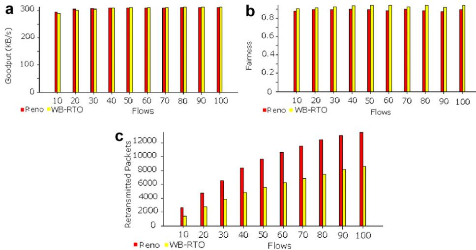
Fig. 15. Protocol Performance, Dynamic Scenario: (a) Goodput (Bytes/s), (b) Fairness, (c) Retransmitted packets.
