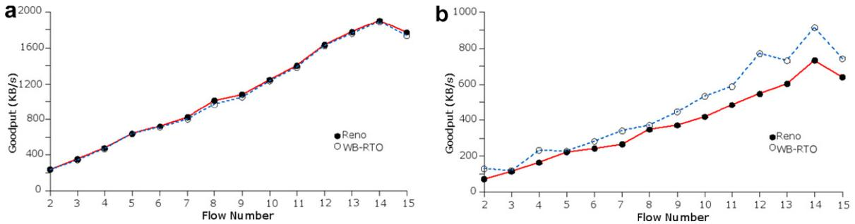
Fig. 7. Goodput performance: (a) No blackout, (b) After three blackouts in 150 s.
